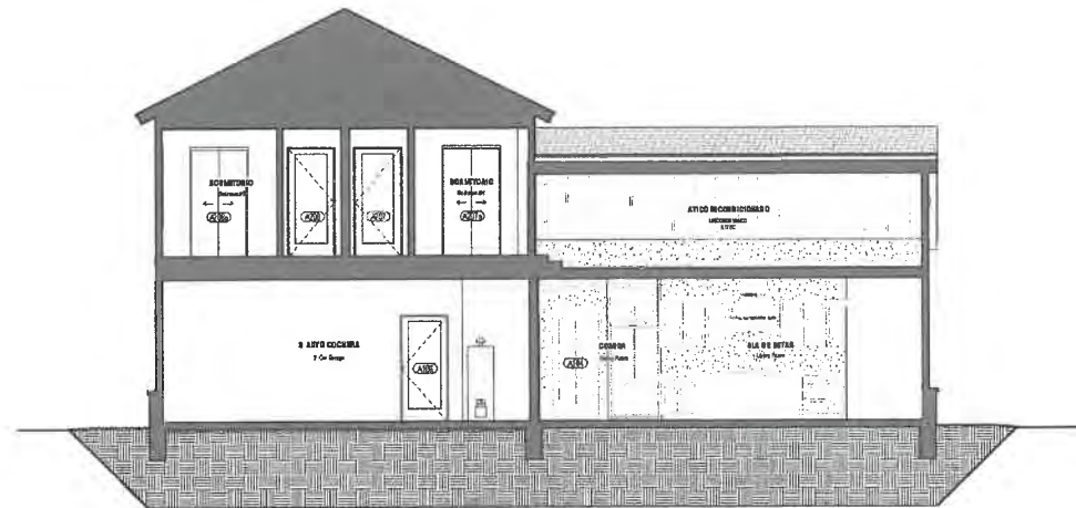
01 | BUILDING SECTION AT GARAGE AND LIVING ROOM 302.000-01-01
