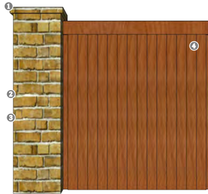
1: Rowlock Cap; 2: Running Bond; 3: 3/8" Tooled Joints (Typical); 4: Wrought Iron or Board-On-Board Wood Fence.
