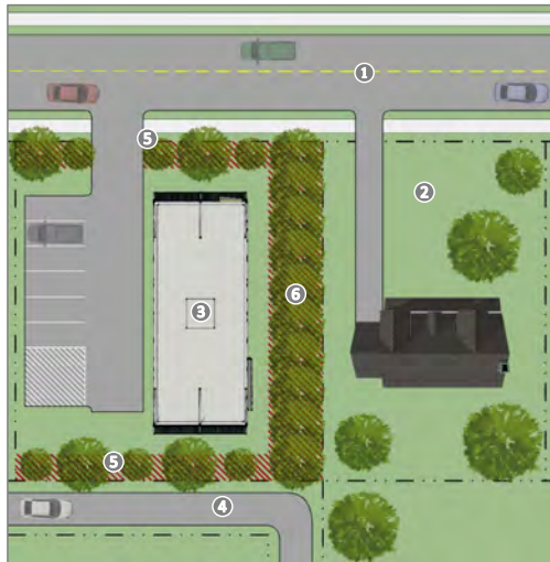
1: STREET; 2: RESIDENTIALLY ZONED OR USED PROPERTY; 3: INDUSTRIAL OR COMMERCIAL ZONING/USE; 4: ALLEYWAY; 5: TEN (10) FOOT LANDSCAPE BUFFER WITH ACCENT AND CANOPY TREES; 6: 20-FOOT LANDSCAPE BUFFER WITH THREE (3) TIERED SCREENING
