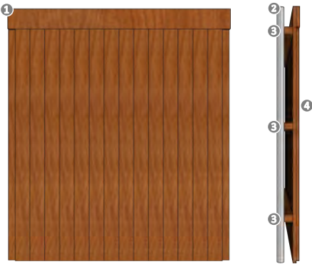
1: Top Rail; 2: Galvanized or Stainless-Steel Post (Recommended Minimum of 2.375"); 3: Stinger Board (Recommended Minimum of 2" x 3"); 4: Minimum 1/2" Wood Screen.
