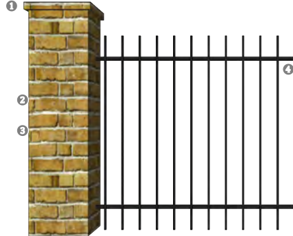
1: Rowlock Cap; 2: Running Bond; 3: 3/8" Tooled Joints (Typical); 4: Concrete Footing/Mow Strip.
