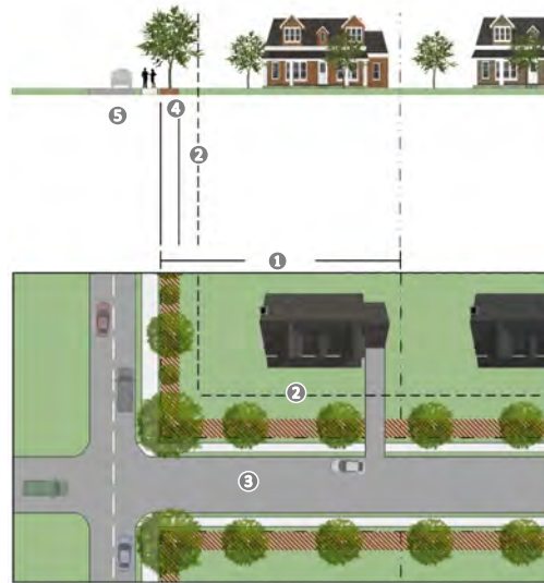
1: RESIDENTIAL PROPERTY; 2: BUILD LINE; 3: COLLECTOR STREET; 4: TEN (10) FOOT LANDSCAPE BUFFER; 5: PERIMETER COLLECTOR OR ARTERIALS ROADWAY
